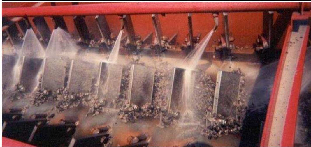
Figure 9: Crushed material enters the logwasher which cleans the material
