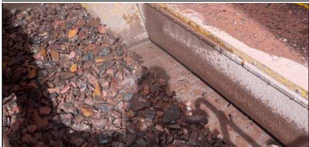
Figure 10: Material is sent to the ore sorter – this material still has too much clay (brown)
